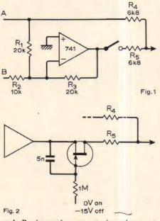
and  $R_4$  (assuming source impedance at input A  $\leq 6.8 k\Omega$ . The degree of attenuation of the unselected input depends on the tolerances of  $R_1$ ,  $R_3$ ,  $R_4$  and  $R_5$ , and if more than about 30dB rejection is required, some trimming may be necessary.
