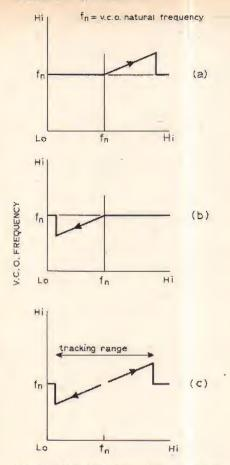
Fig. 17. Tracking range diagram for the p.l.l. (a) reference frequency rising (b) reference frequency falling (c) resultant tracking range.
