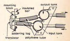
Fig. 1 Mechanical layout of liquid-cooled power output stage
