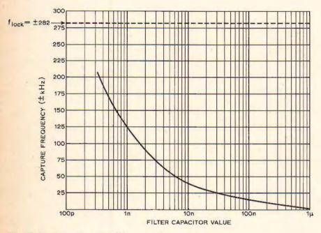
Fig. 20. Capture range versus filter capacitance for 475kHz p.l.l. circuit in Fig. 19. Discriminated output at pin  $7 \approx 100mV$  per 25kHz shift.
