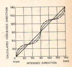
Fig. 4. Perceived localization vs intended direction of sounds in degrees, according to the mid-high frequency theory of this paper, for various systems via a square of speakers as in Fig. 2. Triangles indicate speaker positions. QMX data only applies for a full bandwidth system. Compare with Figs 19 and 20 of reference 26.
