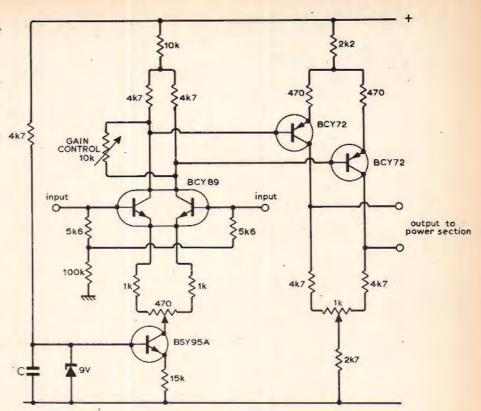
Fig. 7 Preamplifier circuit.
