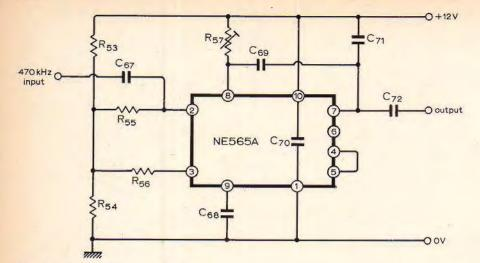
Fig. 19. Practical phase-locked loop circuitry.
