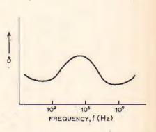
Fig. 8. Loss ongle versus frequency for a polar dielectric material.
