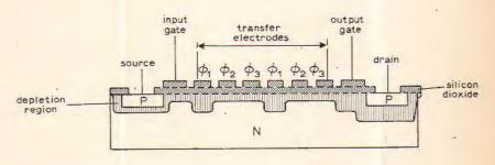
long (in the transfer directions) by  $300\mu m$  wide with a gap between the electrodes of  $2.5\mu m$ .
