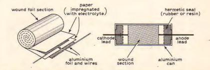
Fig. 11. Construction of an aluminium electralytic capacitor.
