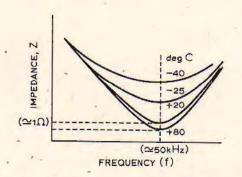
Fig. 4. Impedance curve for a tantalum electrolytic capacitor.
