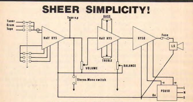
Mono electrical circuit diagram with interconnections for stereo shown
