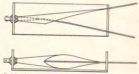
Fig. 5. Coaxial to open-wire flare.
