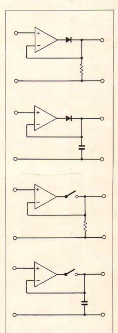
Figs. 1–4. Types of circuit used to measure amplitude of a.c. waveforms (see Table). Complete circuits are given in cards 7 and 8 in set 18.
