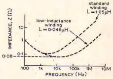
Fig. 5. Impedance reduction obtained by low inductance winding.
