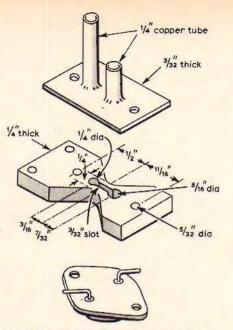
Fig. 4 Dimensions of transistor mountings.
