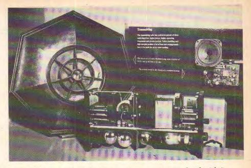
On the left the chassis of a 1923 medium- and long-wave receiver and on the right its present-day equivalent. These are two Philips radio receivers on show in a display covering the story of radio at the newly opened extension of the IBA's Broadcasting Gallery, Brompton Road, Landon.
