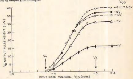
gate voltage determines the hole density in the channel region and so this means that the gate voltage controls or gates the channel current.
