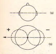
Fig. 1. Omnidirectional and velocity microphones (picture b) receiving the same low frequency information as the human hearing system (picture a). assigning such a sound field to four channels. Similarly, it is not evident, and not in fact true, that feeding these channels directly to a square of speakers gives an optimum recreation of the original sound field.
