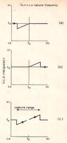
Fig. 16. Phase-locked loop capture range (a) reference frequency rising (b) reference frequency falling (c) resultant capture range. The v.c.o. natural frequency is  $f_n$ .
