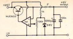
Fig. 12. Circuit of high-current 5V regulator for on-card use.
