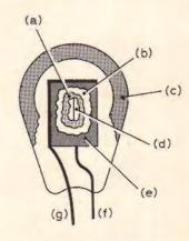
Fig. 13. Schematic of a complete solid tantalum capacitor (a) tantalum impregnated with manganese dioxide (b) graphite layer (c) resin auter coating (d) tantalum shown cut away to indicate anode terminal and tantalum pentoxide layer (e) solder layer completely surrounding cylinder (f) welded anode connection (g) cathode connection.
