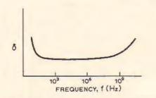
Fig. 9. Loss angle versus frequency for a non-palar dielectric material.
