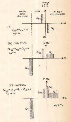
Fig. 9. Schematic diagram of the charge distribution in an m.o.s. structure for three cases: (a) zero volts on the gate, (b) depletion, and (c) inversion.
