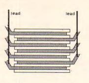
This technique enables high capacitance to be obtained in a relatively small space.
