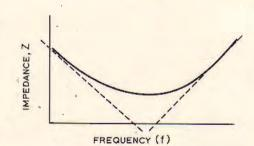
Fig. 3. Impedance versus frequency curve of the simple resonant circuit shown in Fig. 2.
