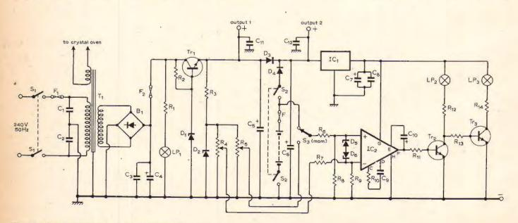
Fig. 11. Main power supply, with battery-condition indicator.
