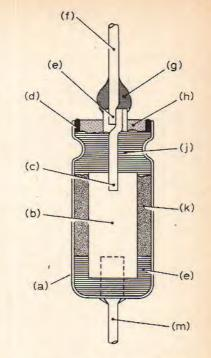
Fig. 14. Schematic of a wet-sintered tantalum capacitor (a) fine silver (b) anodized sintered tantalum anode (c) tantalum wire (d) solder seal (e) tantalum to nickel weld within header (f) nickel wire (g) solder seal between header and external anode lead (h) glass-to-metal seal (j) internal seal (k) electralyte (l) anode boot (m) cathode.
